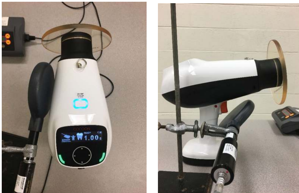
Figure 2. Experimental arrangement of the Cocoon for leakage measurements
